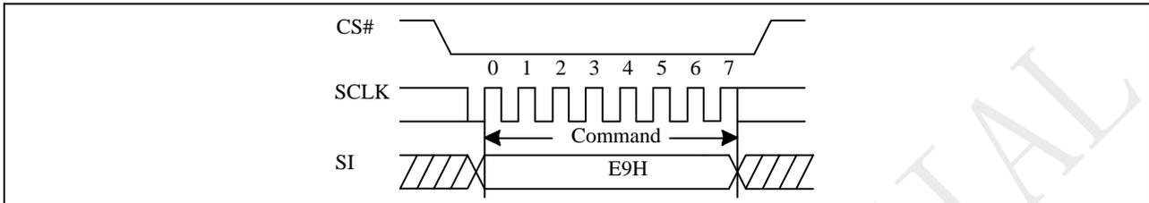
**Figure 10-12a Exit 4-Byte Address Mode Sequence (QPI)**
