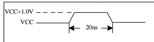
During DC conditions, input or I/O signals should remain equal to or between VSS and VCC. During voltage transitions, inputs or I/Os may negative overshoot to -1.0V or positive overshoot to VCC + 1.0 V, for periods up to 20 ns.
