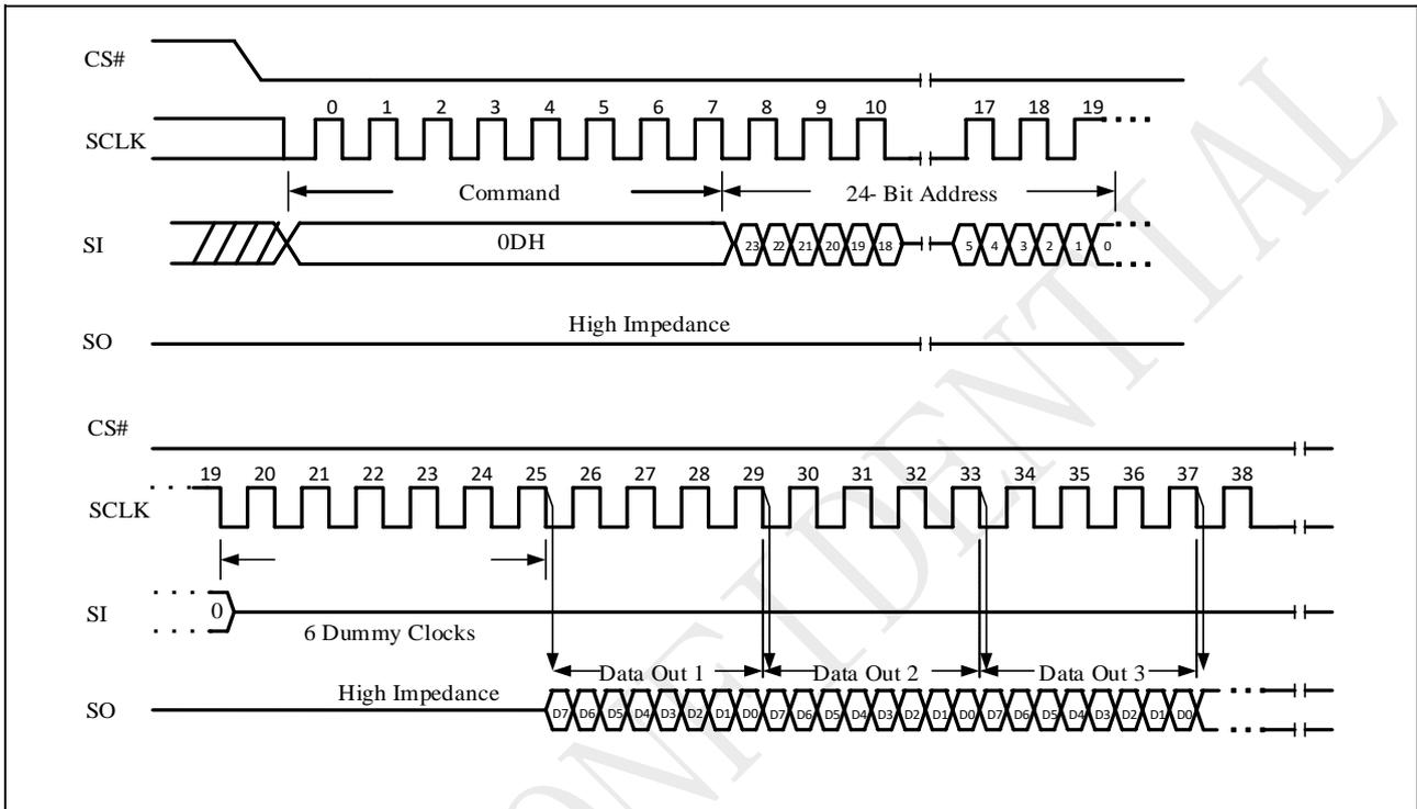
Note: 32-bit address is required when the device is operation in 4-Byte Address Mode. The DTR Fast Read instruction is also supported in QPI mode.
