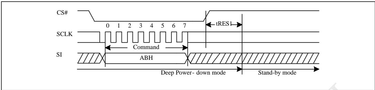
**Figure 10-50c Release from Deep Power-down (RDP) Sequence (QPI)**
