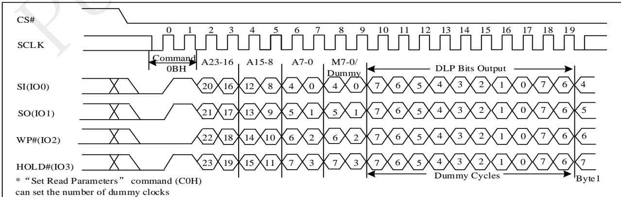
\* "Set Read Parameters" command (C0H) can set the number of dummy clocks
