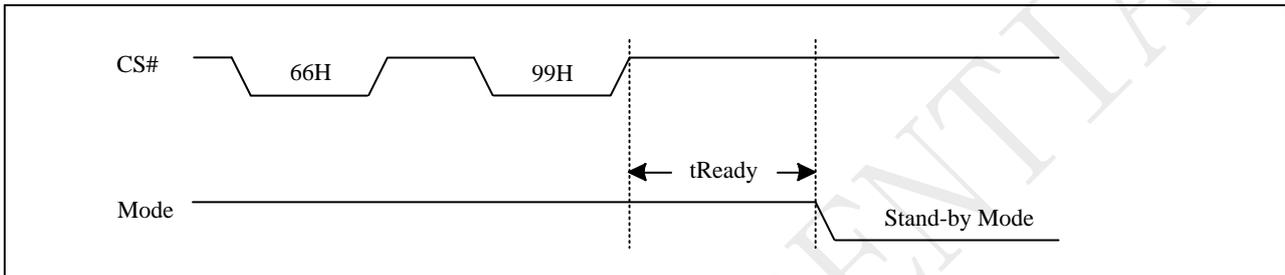
**Figure 10-64a Software Reset Sequence (SPI)**
